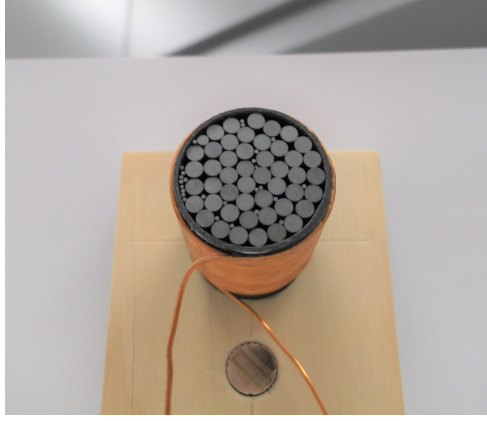
Figure 5.3: Physical structure of the employed ferrite-cored coils.
