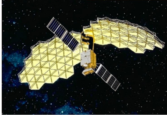
Figure 2.2: Solar panels mounted on a space satellite to transmit microwave power to earth.
