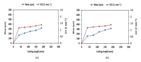
Figure 9. Variation in the SCE with the increase in the tool wear at different cutting lengths for (moderate wear region conditions); (a) Condition 3 ( $V = 130 \,\mathrm{m\,min^{-1}}$ ,  $f = 0.12 \,\mathrm{mm}$  per rev), (b) Condition 8 ( $V = 62.5 \,\mathrm{m\,min^{-1}}$ ,  $f = 0.16 \,\mathrm{mm}$  per rev).
