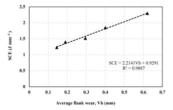
Figure 13. SCE at different flank wear in turning Ti-6Al-4V;  $V = 200 \text{ m min}^{-1}$ , f = 0.12 mm per rev and d = 1 mm.
