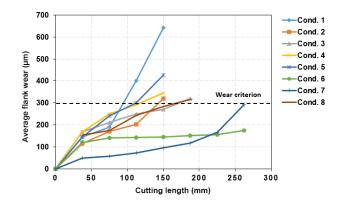
Figure 6. Average flank wear progression vs. cutting length.
