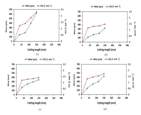
Figure 10. Variation in the SCE with the increase in the tool wear at different cutting lengths for (high wear region conditions); (a) Condition 1 ( $V = 200 \,\mathrm{m\,min^{-1}}$ ,  $f = 0.12 \,\mathrm{mm}$  per rev), (b) Condition 2 ( $V = 125 \,\mathrm{m\,min^{-1}}$ ,  $f = 0.24 \,\mathrm{mm}$  per rev), (c) Condition 4 ( $V = 90 \,\mathrm{m\,min^{-1}}$ ,  $f = 0.24 \,\mathrm{mm}$  per rev), (d) Condition 5 ( $V = 75 \,\mathrm{m\,min^{-1}}$ ,  $f = 0.16 \,\mathrm{mm}$  per rev).
