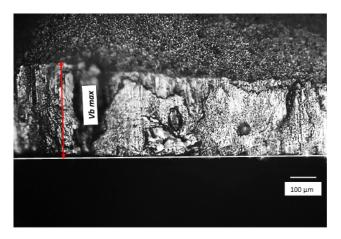
Figure 2. Flank wear measurement using an optical microscope.
