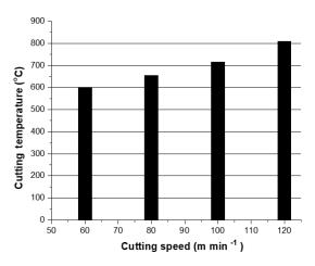
Figure 11. Temperature variation with increasing the cutting speeds (Fan et al., 2016).
