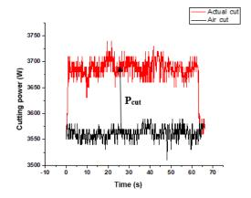
Figure 1. The recorded actual and air cut power to calculate cutting power at cutting condition ( $v = 50 \,\mathrm{m\,min^{-1}}$ ,  $f = 0.12 \,\mathrm{mm}$  per rev and  $d = 1 \,\mathrm{mm}$ ).
