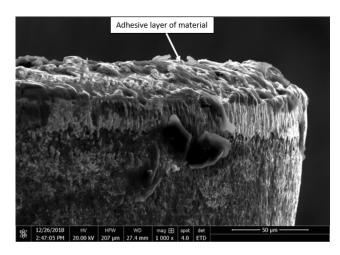
Figure 8. SEM image showing the adhesion of material on rake face at low speed ( $V = 50 \,\mathrm{m\,min^{-1}}$ ).
