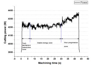
Figure 5. Energy zones during machining titanium (Ti-6Al-4V) alloy at speed,  $V = 200 \,\mathrm{m\,min^{-1}}$ , feed rate,  $f = 0.12 \,\mathrm{mm}$  per rev and depth of cut,  $d = 1 \,\mathrm{mm}$ .
