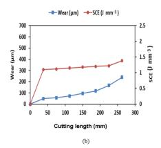
Figure 7. Variation in the SCE due to increase in the wear at different cutting lengths for (low wear region conditions); (a) Condition 6  $(V = 50 \text{ m min}^{-1}, f = 0.12 \text{ mm per rev})$ , (b) Condition 7  $(V = 45 \text{ m min}^{-1}, f = 0.24 \text{ mm per rev})$ .
