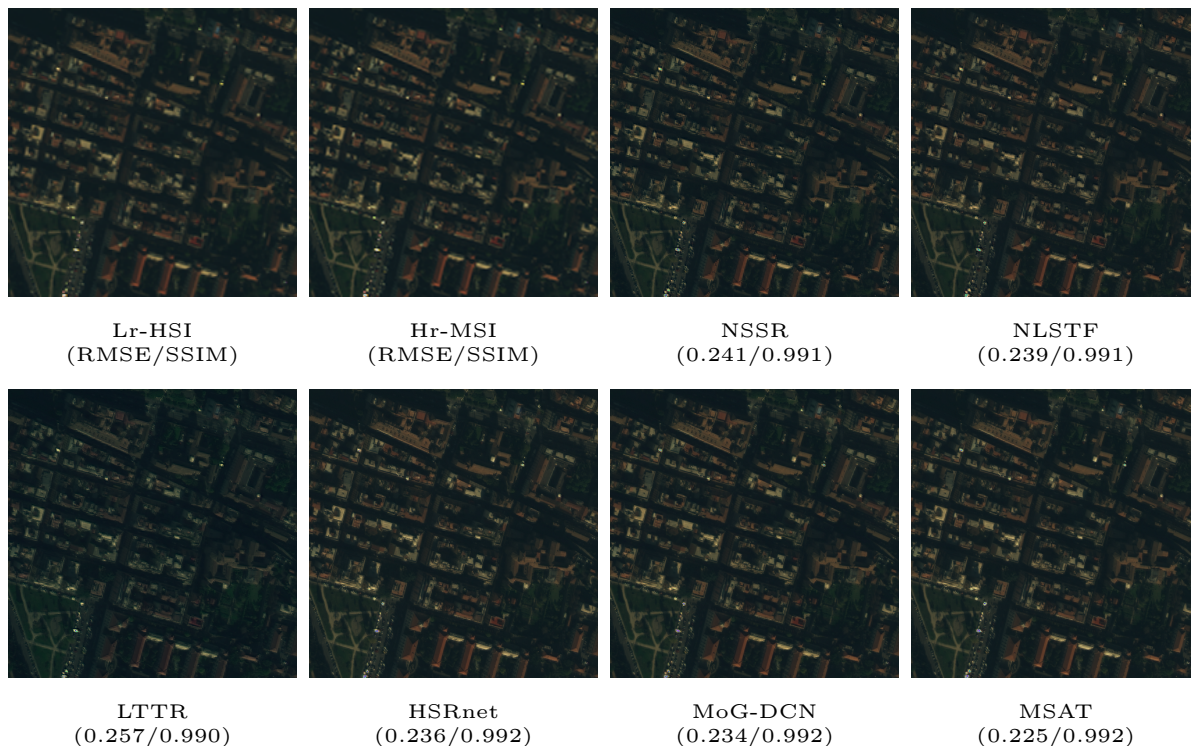
Fig. 9: The Hr-MSI (RGB) and Lr-HSI images are of the left bottom area of Roman Colosseum acquired by World View-2. The composite image of the HS image with bands 5-3-2 as R-G-B is displayed.
