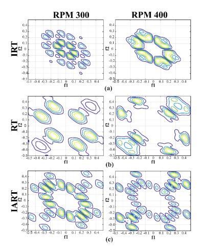
**Figure 14.** Bispectrum visualization of different health types across various speeds: (a) inner raceway type (IRT), (b) roller type (RT), and (c) inner-roller type.
