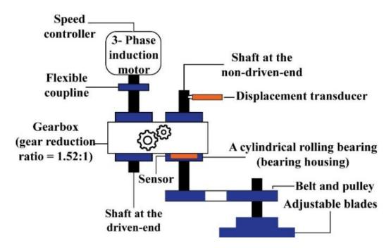
Figure 12. Schematic representation of the self-designed testbed.
