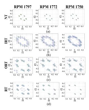
**Figure 6.** Visualization of the bispectra associated with different health types under various speeds: (a) normal type (NT), (b) inner raceway type (IRT), (c) outer raceway type (ORT), and (d) roller type (RT).
