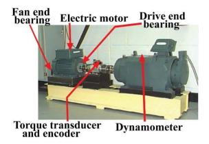
Figure 5. CWRU bearing testbed [71] for collecting vibration signals.
