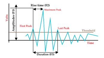
Figure 3. Illustration of AE signal feature.
