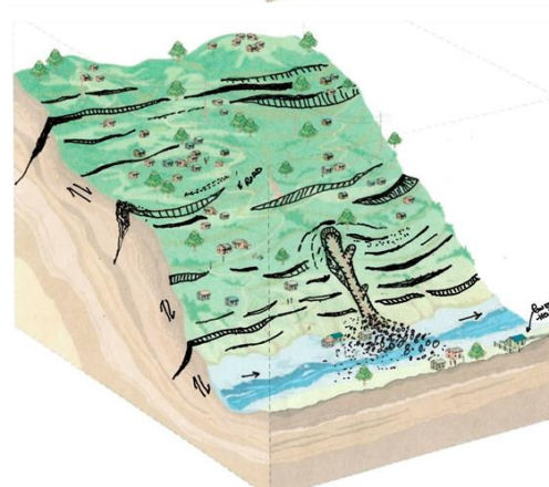
Figure 6-2. Schematic illustration of the landslide demonstrator, showing incremental failure progression. (Base drawing (a) by: C. D. Ranamagar/NSET).
