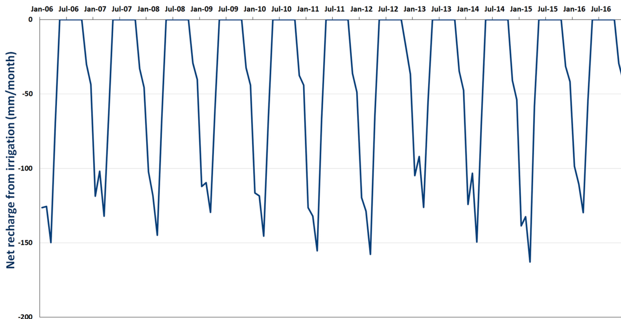
Fig. 19. Time series of mean monthly net recharge to the aquifer from the irrigation during dry season (Nov to April) from 2006 to 2016.
