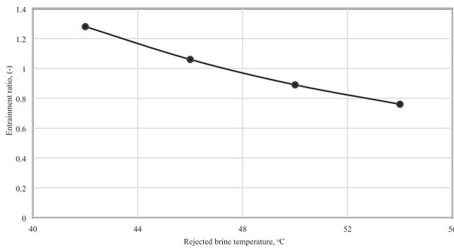
**FIGURE 6** Effect of rejected brine temperature on entrainment ratio at fixed top brine temperature (TBT) of 60°C
