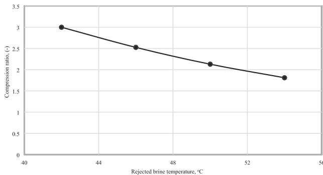
**FIGURE 7** Effect of rejected brine temperature on compression ratio at fixed top brine temperature (TBT) of 60°C
