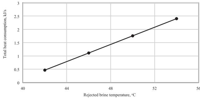
**FIGURE 4** Effect of rejected brine temperature on total heat consumption at top brine temperature (TBT) of 60°C
