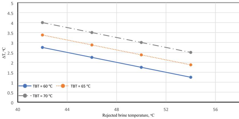
**FIGURE 3** Variation of the temperature drop between the effects when the rejected brine temperatures are varied at different top brine temperatures (TBTs)
