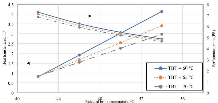
**FIGURE 2** Effect of rejected brine temperature on performance ratio (PR) and heat transfer area at different top brine temperatures (TBTs)
