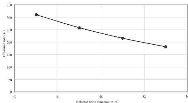
**FIGURE 8** Effect of rejected brine temperature on expansion ratio at fixed top brine temperature (TBT) of 60°C
