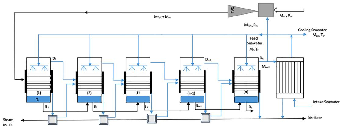
FIGURE 1 Parallel multi-effect distillation with thermal vapour compression (MED–TVC) system with  $n$  number of effects
