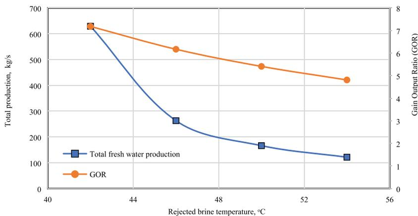
**FIGURE 5** Effect of temperature of the rejected brine on total freshwater production and gained output ratio (GOR) at top brine temperature (TBT) 60°C
