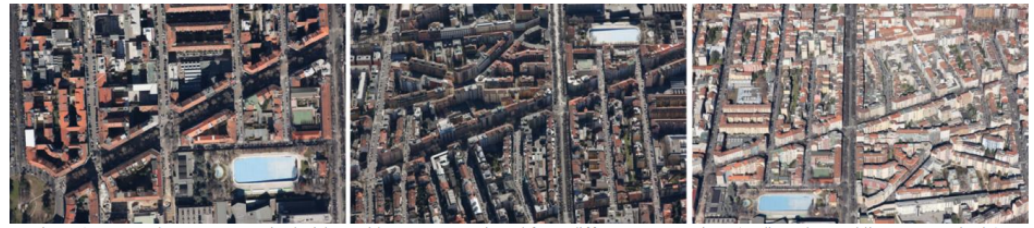
Figure 9. Left: nadir, middle and right: oblique views of the same urban scene. The differences in radiometric resolution between the views, cause difficulties in image matching. Reprinted with permission from Ref. [77].
