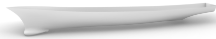
Figure 5: DTMB 5415 hull model used as a test case for the proposed approach.
