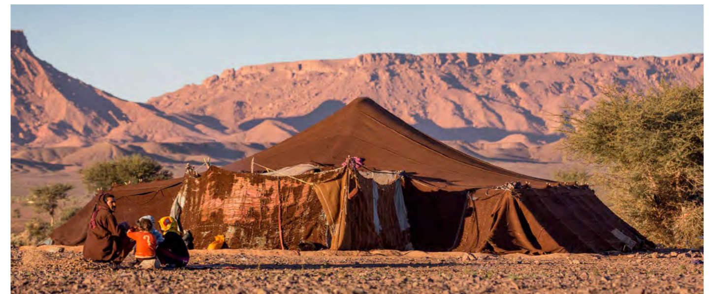
Figure 3 – The best cloth forms the roof where tensions are greatest. Berber Tent, Morocco. Gordon Clarke, 2016
