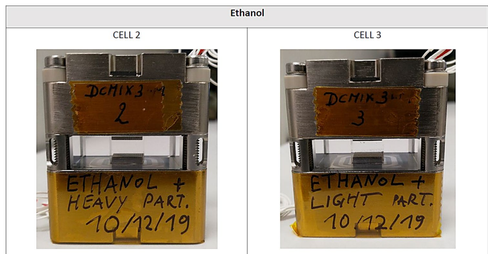
Fig. 18 Cells filled with ethanol and different particles types used for the long-duration compatibility tests
