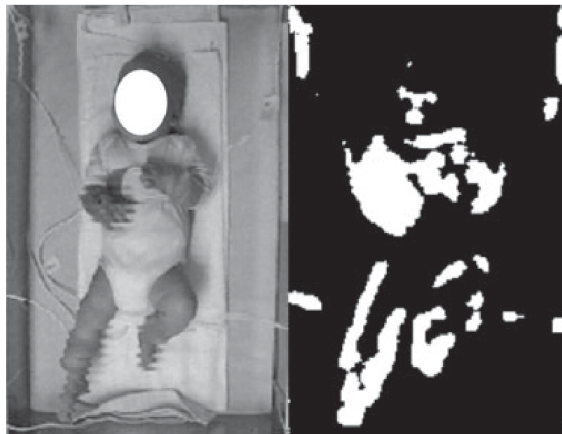
Figure 2.8: Frame differencing example. In the image on the right, pixels displayed in black indicate no movement occurred between the frames, pixels displayed in white represent movement [128]
