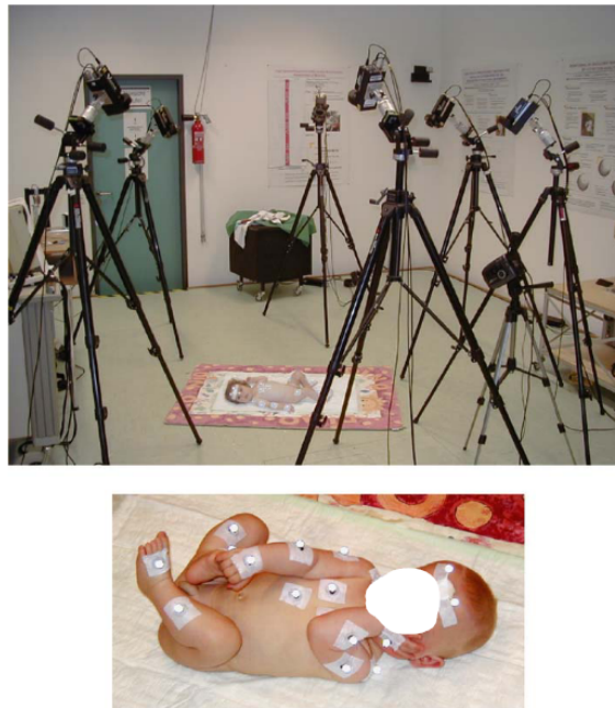
Figure 2.7: Motion analysis system, measurement setup and marker placement [112]
