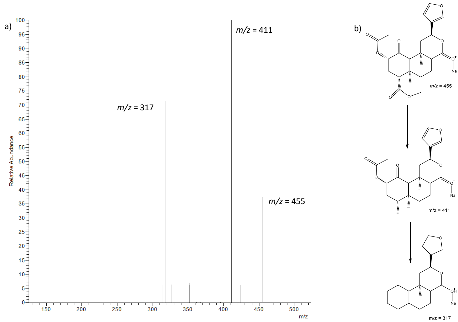
Figure 6.16: Full scan MS/MS spectrum for a) salvinorin A and b) compound fragmentation
