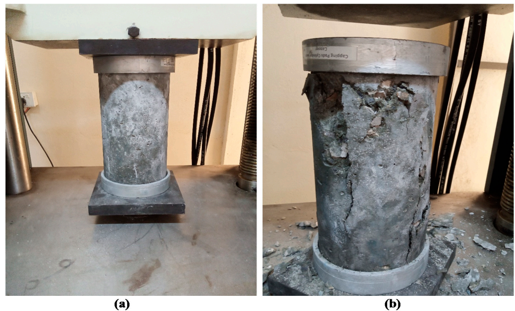
Figure 7. Compression test assembly: (a) cylinder before test and (b) cylinder after test.
