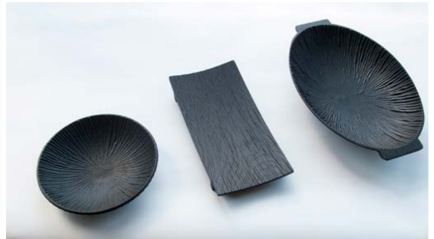
Figure 1. Marshall's 'Hand Thought' series of CNC milled oak tableware (2018). From left to right: Small bowl 210x45mm; Japanese platter 230x120x40mm; Oval dish 370x260x60mm.
