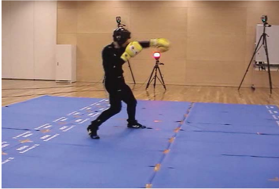
Figure 3.2: Motion capture on a single human. The shadow boxing motions of several boxers were captured using an optical motion capture system.
