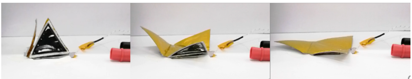
Figure 12. Sequential deployment of the pyramid sample with an external flat heater on the base
