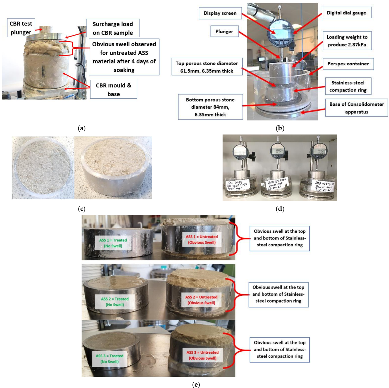
Figure 6. (a) Swell observed after soaking CBR untreated ASS samples; (b) consolidometer apparatus used in this study; (c) compacted swell samples in stainless-steel compaction ring; (d) swell set-up for treated and untreated ASS materials; (e) treated and untreated ASS samples after the swell test.
