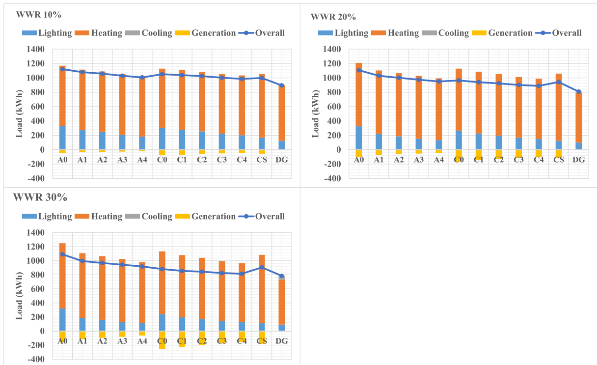
Fig. 2. Overall Energy Performance for small glazing.
