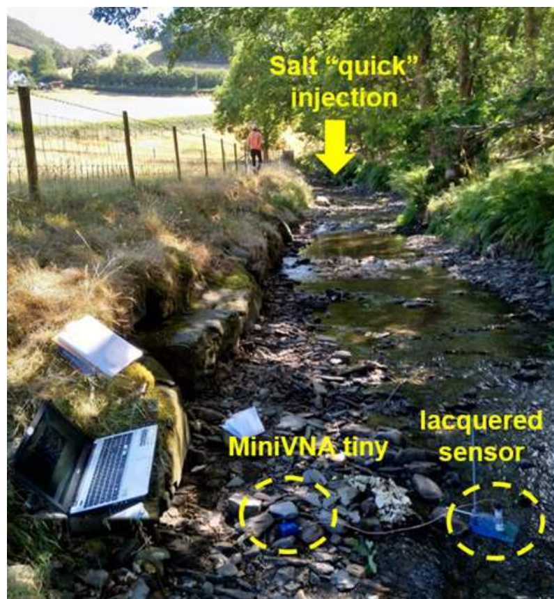
Figure 7. Evaluation of the feasibility to measure “unexpected” variation in a parameter (NaCl in this case) in freshwater and the return to the baseline level.
