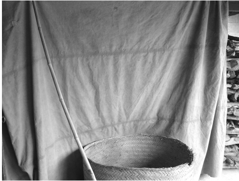
Figure 7. Further optimisation of the recording environment. A piece of thick, rough cloth is used to cover sound-reflecting surfaces and open space, which also dampens background noise.
