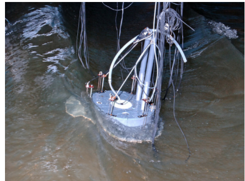
FIGURE 5. MODEL OF THE CALM BUOY IN THE SHALLOW WATER BASIN AT MARIN
