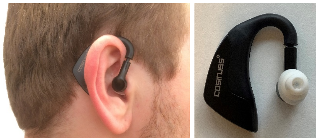
Figure 1. The wearable ear thermometer Cosinuss° °Temp. Left: Cosinuss° position in the ear. Right: Cosinuss° with IR sensor in the white ear tip.
