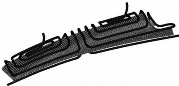
Fig. 11. A design consisting of two sub-CC channel systems (Reprinted by permission from [64], Copyright 2009 KSAE and Springer).
