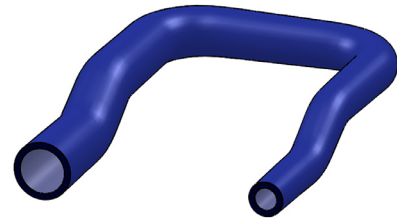
Fig. 7. A design of a variable diameter CC channel.
