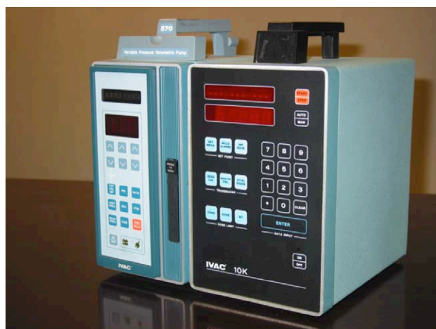
Figure 2. Picture of the IVAC titrator (Becton, Dickinson, and Company, San Diego, CA), the first electronically controlled infusion pumps with fluid flow technology. The photograph is courtesy of Bob Butterfield, used with permission from Becton, Dickinson, and Company (San Diego, CA).
