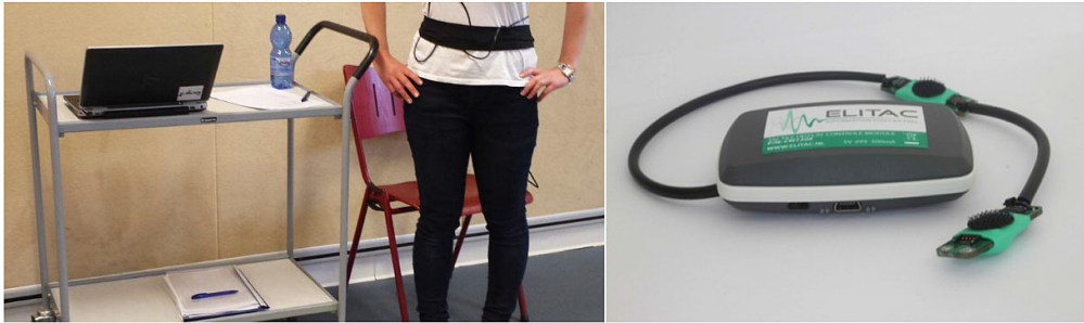
Fig. 1. Participant wearing the tactile belt over a T-shirt (left) and a control unit with two factors (right).
