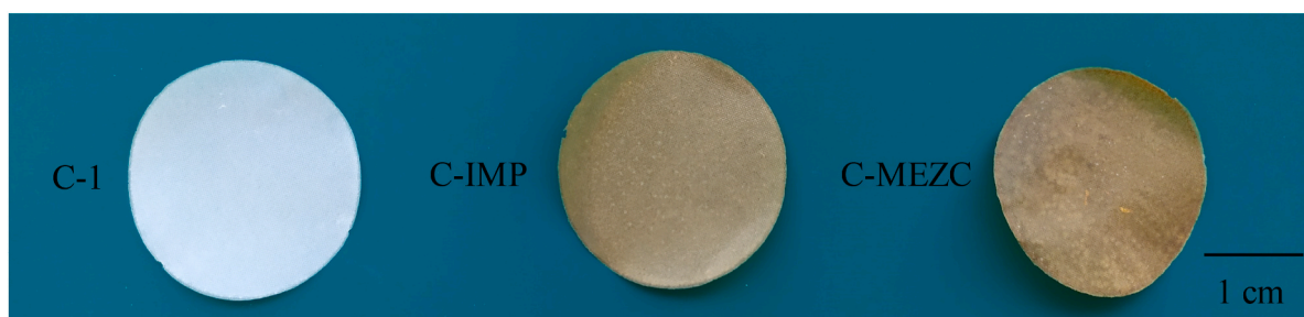
Fig. 3. Photograph of MFC membrane (C-1) and composite membranes prepared by solution impregnation (C-IMP) and solution mixing (C-MEZC).
