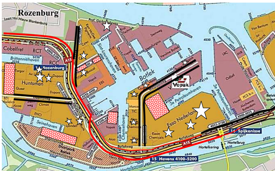
Fig. 1. Botlek area with industrial plants emitting CO 2 (white stars). The size of the white stars reflects the annual amount of CO 2 emissions. The red-dotted rectangular denote the possible space available for CO 2 capture installations and additional energy plants. A simplistic overview of the pipeline strips is indicated by the red and black lines; the black lines indicate the pipeline strips in which (practically) no space is available for new (large diameter) pipelines, while the red lines indicate the pipeline strips in which space is still available (Pipelinex, 2012a,b,c). The high pressure trunk CO 2 pipeline planned by the Rotterdam Climate Initiative would roughly follow the track of the black–white line on the map. (For interpretation of the references to color in this figure legend, the reader is referred to the web version of this article.)
