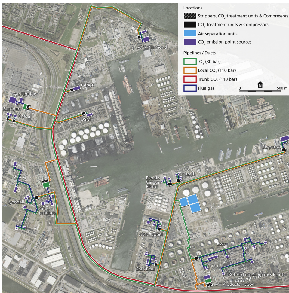
Fig. 10. Aerial photograph of the industrial Botlek area with the Oxy-Hybrid (EI) configuration.
