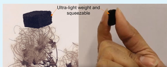
Ultra-light weight and squeezable graphene-PDMS foam for piezoresistive sensing
