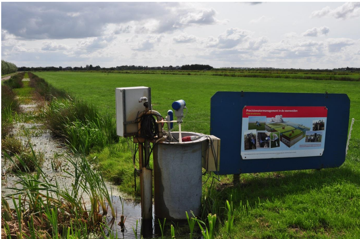
Experimental pressure drainage in a peat meadow in the Netherlands. Photo: Hans Joosten.
