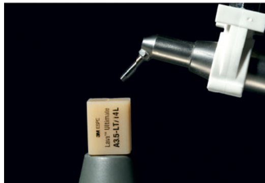
Fig 3 Standardization of airborne particle abrasion via a special apparatus.
