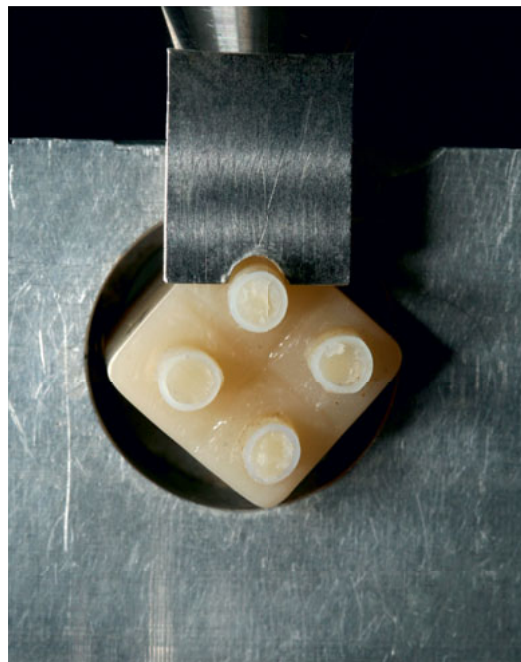
Fig 4 Shear bond testing.
