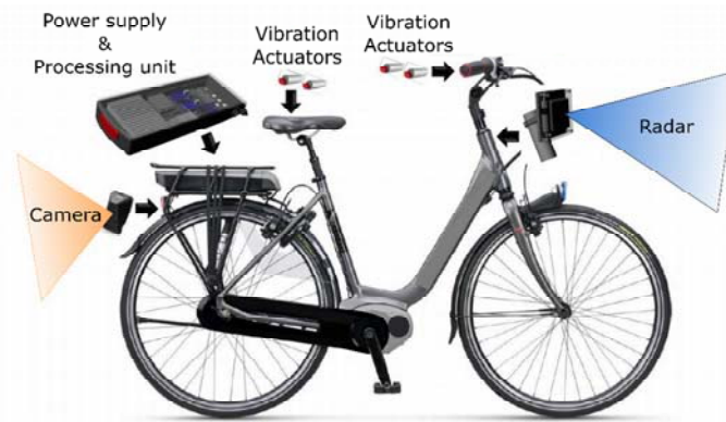
Figure 1 Instrumented bicycle with components that was used during the experiment (see online version for colours)
