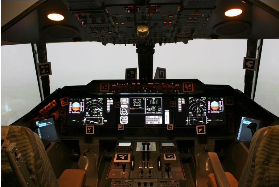
Figure 5. Touchscreen HMIs integrated in full-motion flight simulator GRACE
