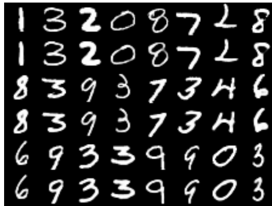
Figure 11: Image encoding and reconstruction for the MNIST dataset. Rows 1, 3, and 5 are the original images taken from MNIST, rows 2, 4, and 6 are the corresponding reconstructed images based on the encoding. The used networks are described in Table 1, trained with WGAN-GP.
