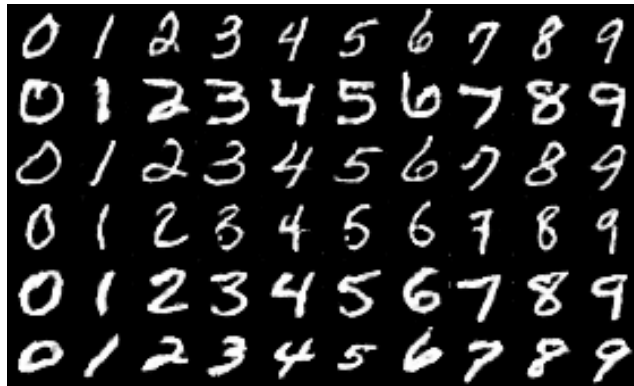
Figure 9: Random samples for MNIST, conditioned on digit label. Every column corresponds to a unique label, the samples in a row have the same latent noise vector. The used networks are described in Table 1, trained with the conditional WGAN-GP.
