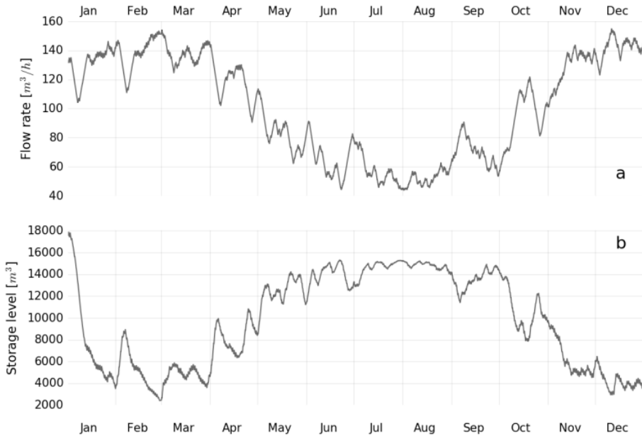
Figure 7.4: Geothermal system flow rate (a) and corresponding storage level (b) for a re-injection temperature of 40^\circ\text{C} .
