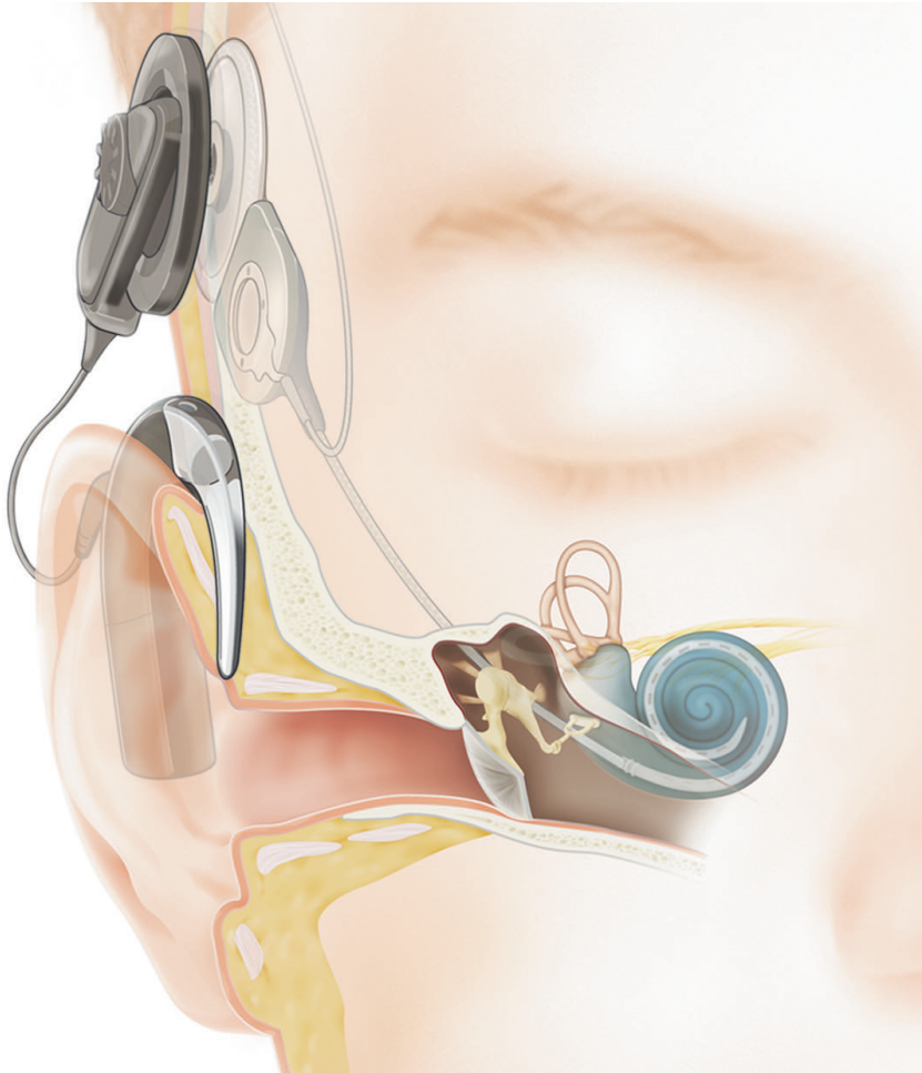
Figure 1: Illustration of a right ear with a cochlear implant. Hooked behind the ear (or pinna) is the speech processor, which connects to the transmitter that sits on the skull (dark gray). The transmitter is held in place by a magnet that connects it to the receiver embedded in the skull (translucent), which in turn connects to the electrode array inserted in the cochlea. Image Copyright Cochlear Limited ©
