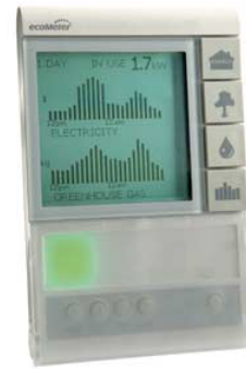
Fig. 1. A typical IHD interface, the ecoMeter, displaying a green "safety" light [11].
