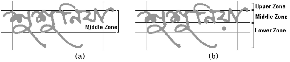
Fig. 7. For the word image “SHUSHUNIA”, (a) middle zone detected by \alpha_i , (b) zones detected by \alpha'_i .
