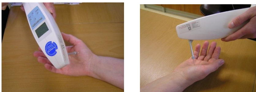
Figure 6, 7. Myometer for muscles stiffness measurements
