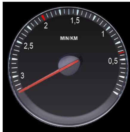
Figure 1. Pace meter indicating the inverted speed in minutes per kilometre.
