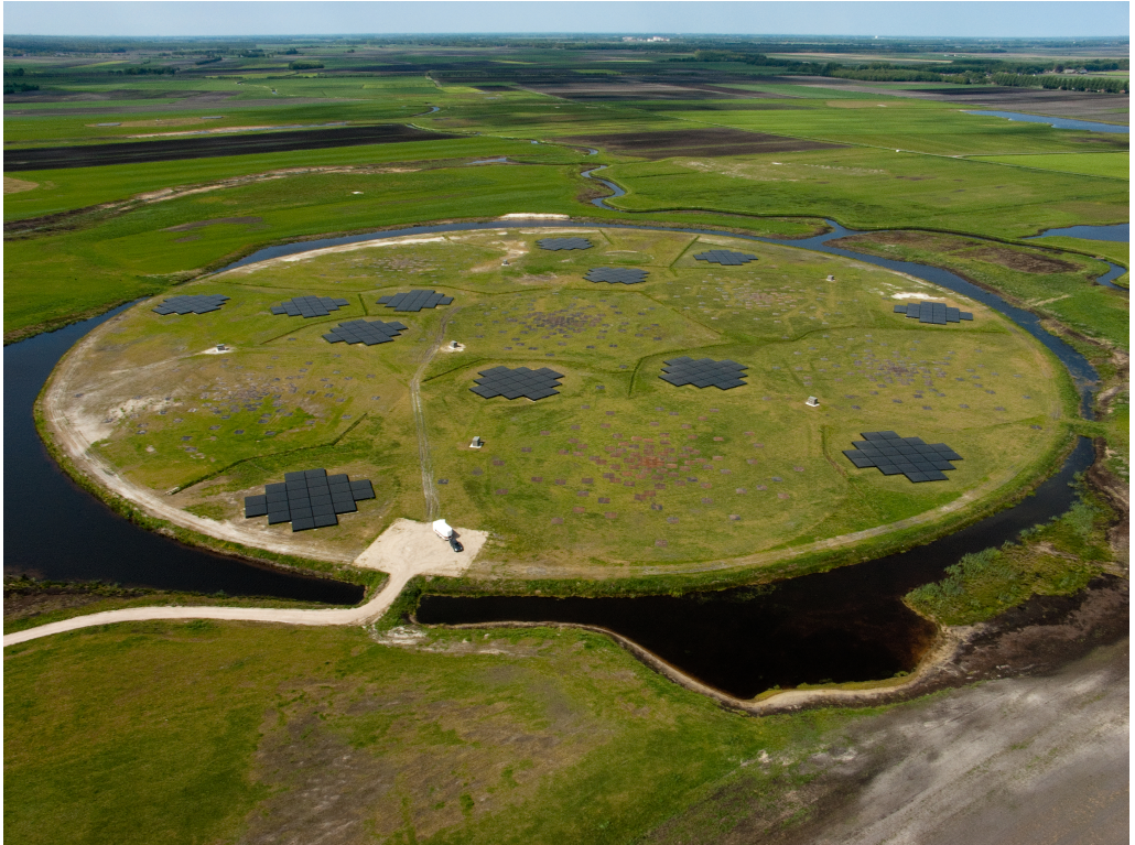
Figure 3: The six stations comprising the very core of the LOFAR telescope, the so called super-terp imaged on May 23, 2010 (© Top-Foto, Assen).
