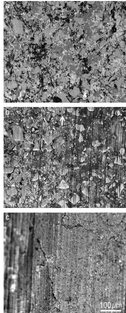
Fig. 6. Light micrographs showing the wear evolution of the same area on a worn surface ( \phi 22 mm) on the Epomet-PTFE-20 sample, sliding against the \phi 13 mm 100Cr6 steel ball at 60 N load and 2 cm/s speed, after various sliding distances: (a) 0 m (original surface), (b) 400 m and (c) 1000 m. The arrow indicates the relative sliding direction of the counterpart steel ball.
