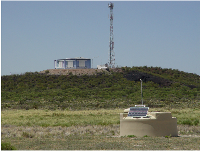
Figure 5.1: The Los Leones fluorescence telescope with on the foreground one of the water tanks of the surface detector at the Pierre Auger Observatory.
