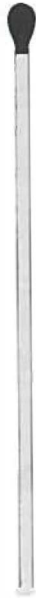
Fig. 13 Glass capillary, filled with cervical mucus. By pressing the plug of modelling wax a short way into the glass capillary, some cervical mucus protrudes from the other end.
