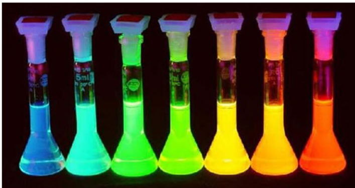
Figure 1.2: Size dependent fluorescence. Photograph of solutions of 2 to 7 nm CdSe nanocrystals, with increasing diameter from left to right. The semiconductor band gap increases with decreasing nanocrystal size, leading to a color shift from red to blue. [2]
