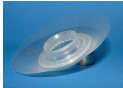
Figure 3. The silicone rubber based tracheostoma patch has a thin flexible conical base.
