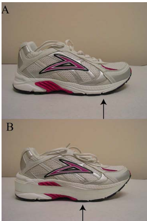
Figure 1. Investigated shoes in this study: (A) standard running shoes, and (B) rocker shoes. The black arrows indicate the shoe apex (rolling-point).
