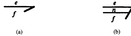
Fig. 5. A bond with effort variable e and flow variable f . (a) Single bond. (b) Multibond.
