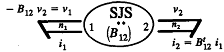
Fig. 8. Simple junction structure representing the fundamental loop matrix B = (I_{n_1 \times n_1} \ B_{12}) .
