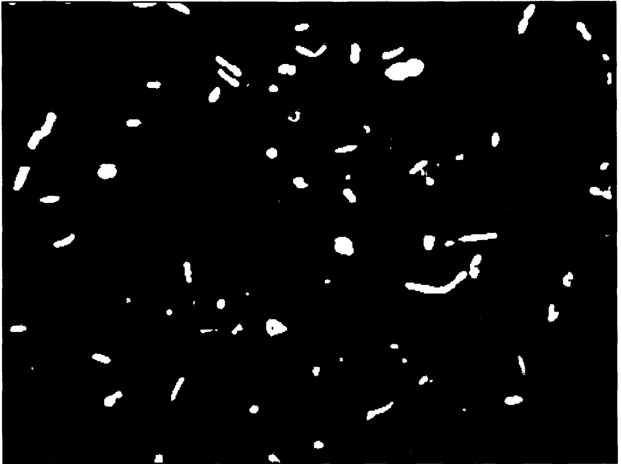
Fig. 1. A typical binary image of a full field of view of bacteria, as acquired and segmented by the morphometrical program of our image processing system.
